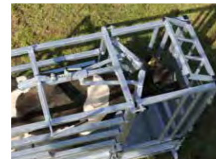
6. MANUAL HEAD YOKE Saloon style locking doors
