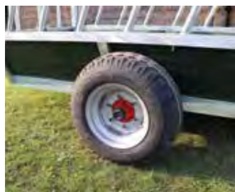
10.0 75 X 15.3 6-STUD WHEELS ON 60MM STUB AXLES
