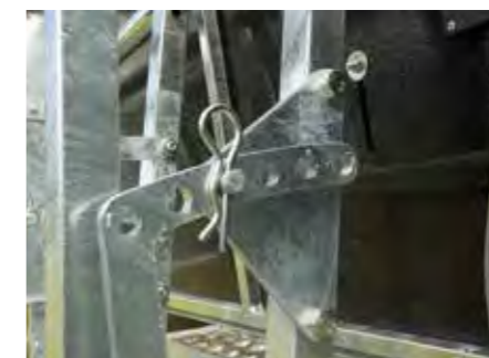
9. WIDTH ADJUSTMENT Quick adjustment to the grip width
