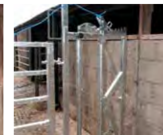
WIDTH ADJUSTMENT ON YOKE APERTURE
