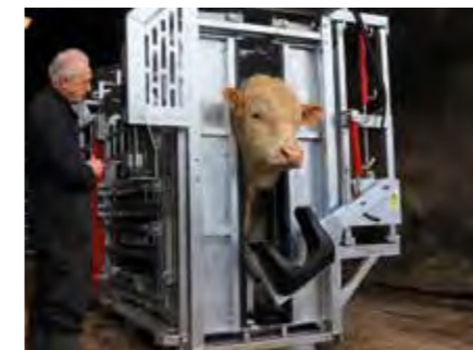
6. HYDRAULIC HEAD RESTRAINT Dedicated twin lever operated control valve for pivot and lift functions
