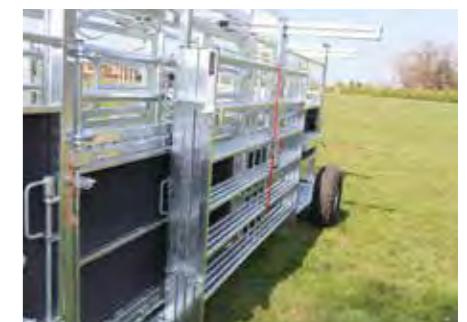
11. CATTLE HURDLE TRAVEL HOOKS AND STRAPPING For safe transportation of the hurdles
