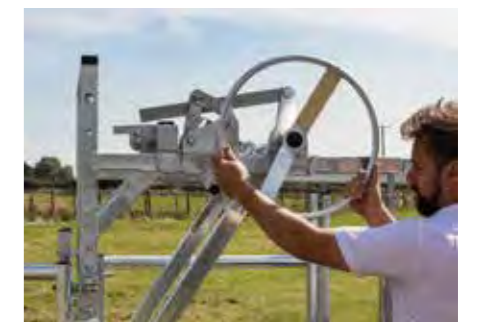
8. DROP DOWN RUMP BAR Revolving ratchet style rump bar
