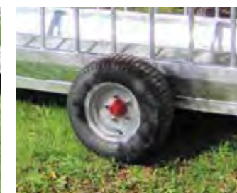
23 X 10.5 -12 5-STUD WHEELS ON 50MM STUB AXLES
