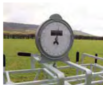
MECHANICAL VERSION COMES WITH 100KG WEIGH CLOCK
